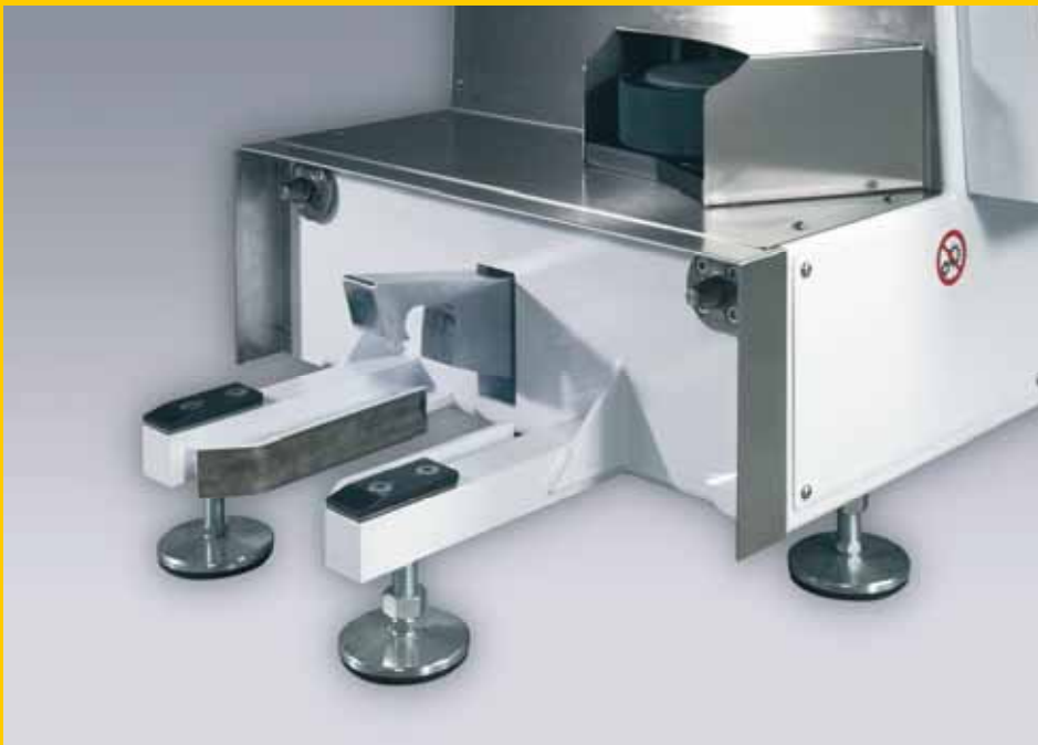
Hydraulic hooking and lifting mechanisms
